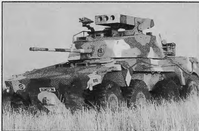
Rooikat 35/ZT3 Tank Destroyer — version of Rooikat 35 equipped with pod of three ZT3 Swift laser-guided antitank missiles. Nine more missiles are carried in reserve.
